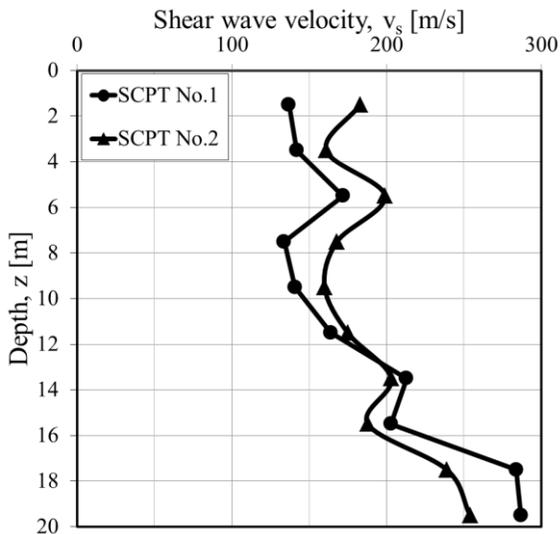
Figure 2. Shear wave velocity profiles of the site.
